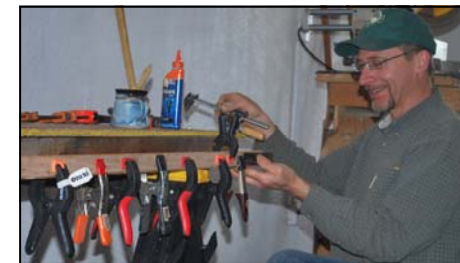
Mike Hubbard made a laminated paddle, which required several flat pieces of different kinds of wood glued together.
